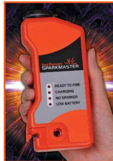
The SparkMaster cannot be operated without the magnetic key and firing can be aborted simply by releasing the magnetic key and allowing it to be ejected by the spring-loaded mechanism. The main capacitors will discharge internally returning it to a 'safe' condition.
